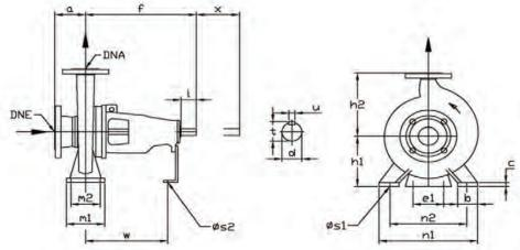
Fig. 2.2 – End-Suction Pump Drawing
