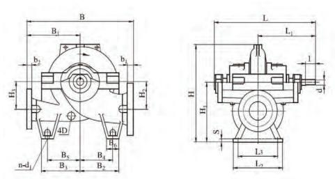
Fig. 1.2 - Split-Case Pump Drawing
