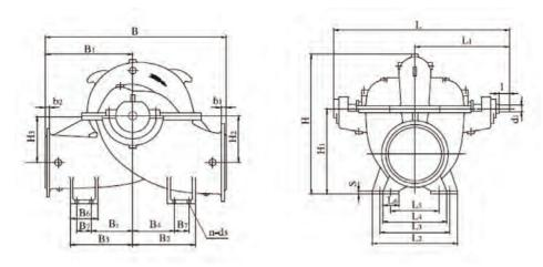
Fig. 1.3 – Split-Case Pump Drawing
